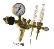
The cylinder pressure regulator with manual connection reduces the cylinder pressure of compressed gases and gases dissolved under pressure of max. 200 bar (300 bar on request) to a pressure corresponding to the flowmeter. The desired flow rate in I/min can be constantly set on the flowmeter.
